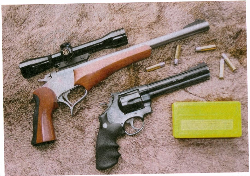
Comparing the .44 Magnums: A Contender pistol (top) and a Smith & Wesson Model 29 Hunter, both in .44 Mag. The revolver has capacity, but with a longer barrel and fixed breech, the Contender can be more accurate and easily adaptable to optical sights.
