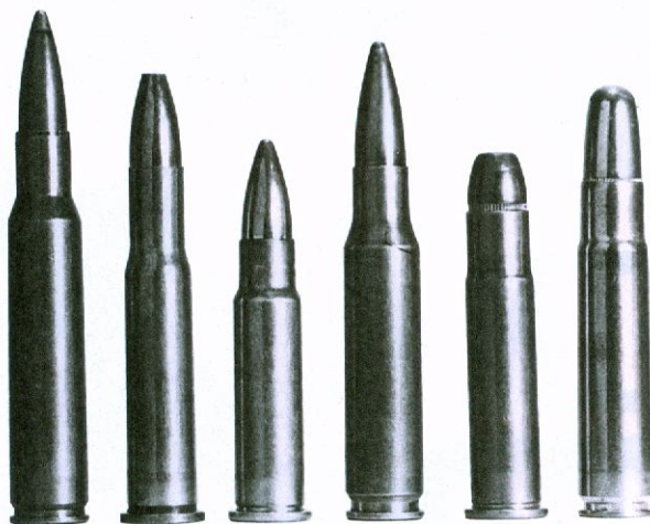
Left to right: 7x57 Mauser, .30-30 Win., .30 Herrett, .308 Win., .357 Herrett, .35 Rem. The Herrett wildcat cartridges, based on the .30-30 case shortened with body taper reduced, were designed to maximize performance with fast-burning powders in 10-inch Contender barrels.
